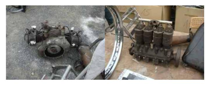
Two interesting engines. Left - A BMW based stationary engine. Right - An early FN four cylinder.
